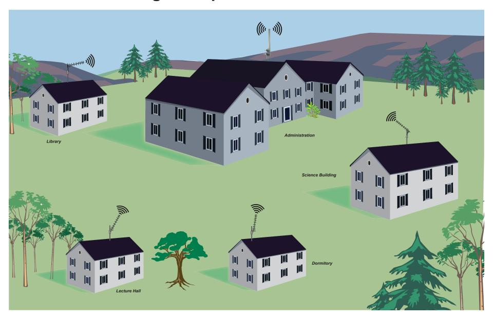
This application diagram represents a typical point to multi-point wireless network used in a campus environment. The central Administration building utilizes an Omni directional antenna and the satellite buildings use directional Yagi antennas for bi-directional communication with the Administration building.
