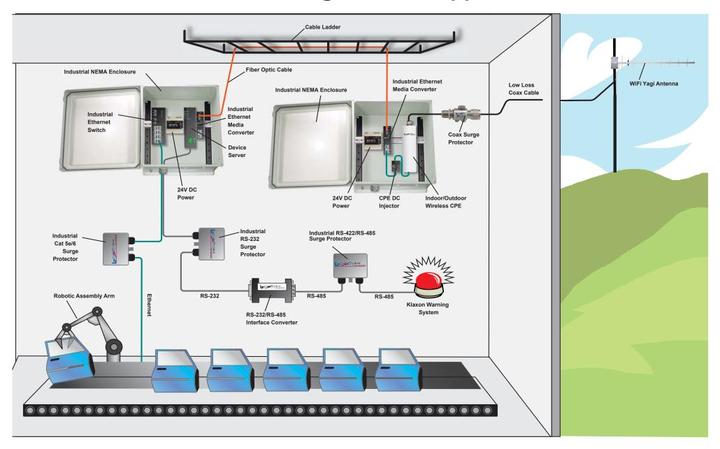
This diagram is representational only and depicts a typical manufacturing network application. The diagram encompasses Ethernet, RS-232, RS-485, and WiFi connectivity to provide an end to end manufacturing network solution.
