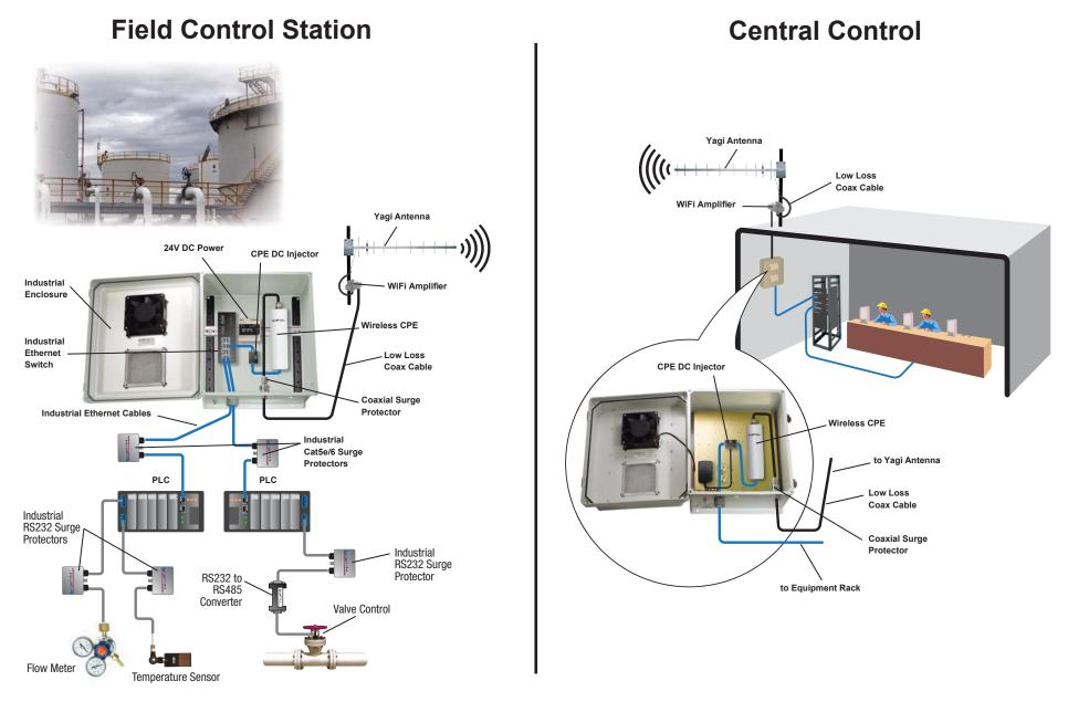
This diagram is representational only and depicts a process automation network. The diagram encompasses Ethernet, RS232, RS485 and WiFi connectivity to provide an end to end process automation networking solution.
