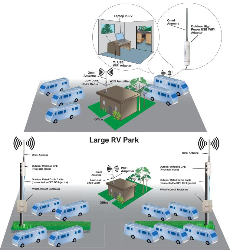
This diagram is representational only and depicts a typical RV Park WiFi application. Each wireless installation is unique and results can vary due to many different environmental factors. For outdoor wireless networks Line of Sight (LOS) must be considered. Basically that means you will need a clear unobstructed view of the antenna from the remote point in the link. Trees and leaves are obstructions to 802.11 frequencies so they will partially or entirely block the signal.
