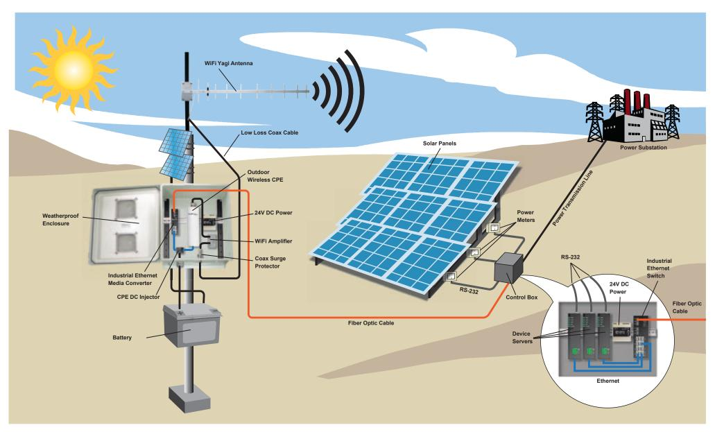
This diagram is representational only and depicts a typical solar energy network application. The diagram encompasses Ethernet, RS-232, and WiFi connectivity to provide an end to end solar energy networking solution.
