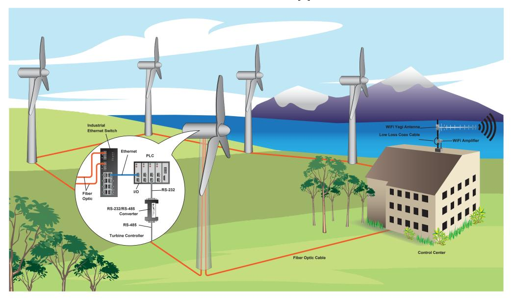
This diagram is representational only and depicts a typical wind farm network application. The diagram encompasses Ethernet, RS-232, RS-485 and WiFi connectivity to provide an end to end wind energy networking solution.
