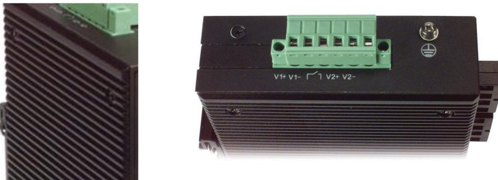
The image on the left details the case of an Industrial Ethernet Switch that acts as the heat sink for the unit. The image on the right shows dual power inputs as well as a dry contact for connecting alarm devices for visual or audio warning in the event of a power supply failure.
